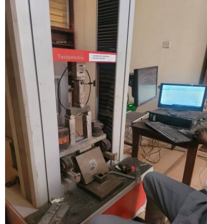
Figure 3: Flexural Strength Test Setup
