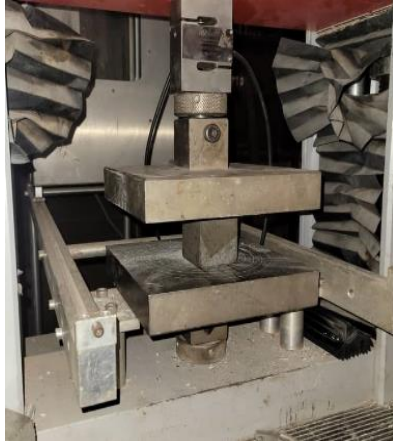
Figure 2: Compressive Strength Test Setup
